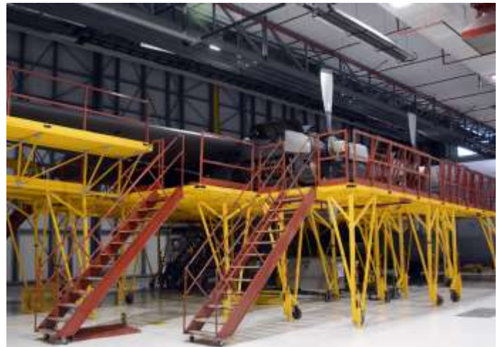
A portion of 12-pieces of C-130 Hercules exterior access maintenance stands provided by Dyess Air Force Base are assembled in the 120th Airlift Wing's main hangar in Great Falls, Mont., on Jan. 30, 2015. (Montana Air National Guard photo/Senior Master Sgt. Eric Peterson)
